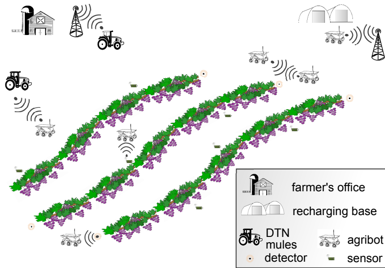
Figure 3: Precision viticulture in a Delay Tolerant Network environment
